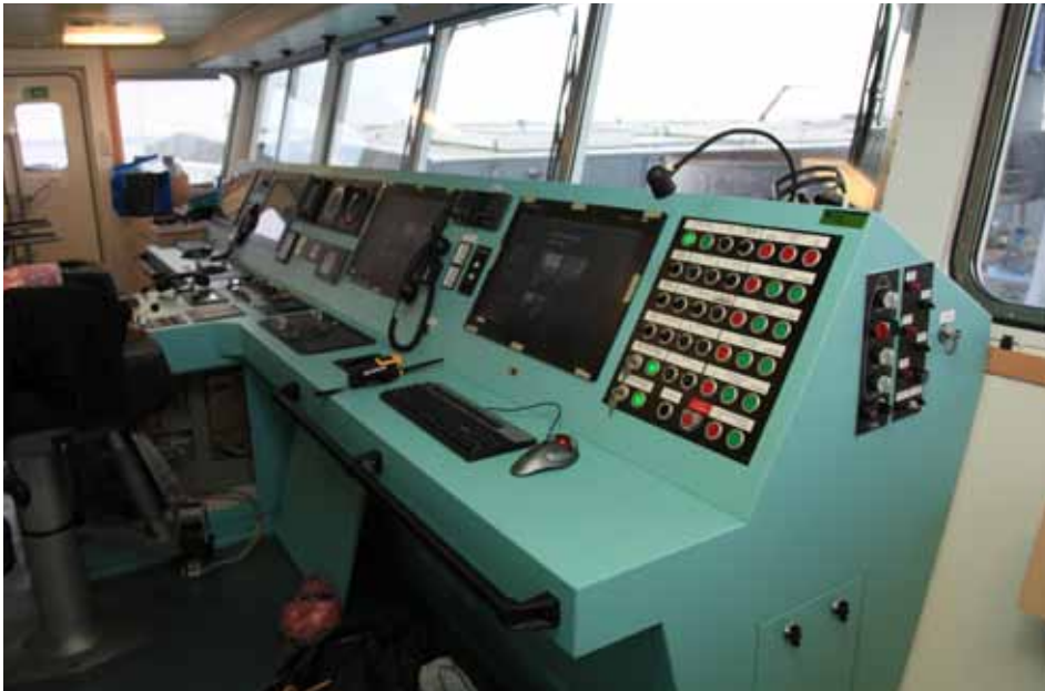
* The wheelhouse forward area contains the T-shaped navigation console by SAM Electronics
