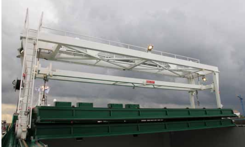
* Handling of all hatch panels is done with a Coops & Nieborg gantry crane on coaming rails
