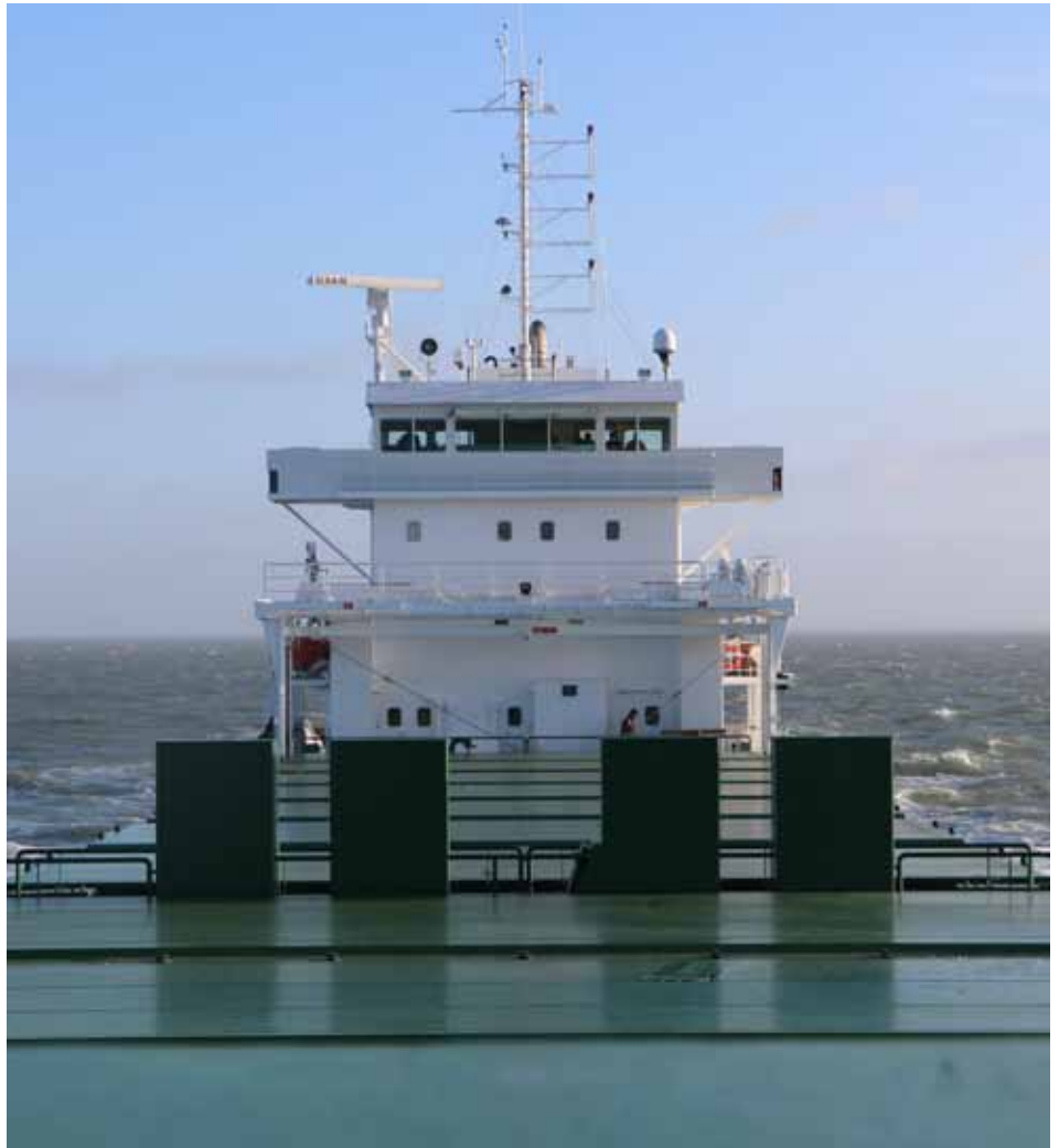
* The upper deck, with closed hatch covers and the ventilation equipment on top of the hold separation
