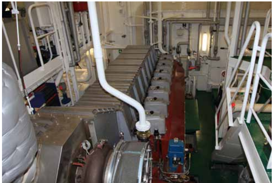
* A single Berg CPP is powered by a MaK marine diesel engine via a JaKe gearbox
